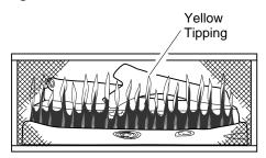
Figure 42 - Incorrect Burner Flame Pattern
